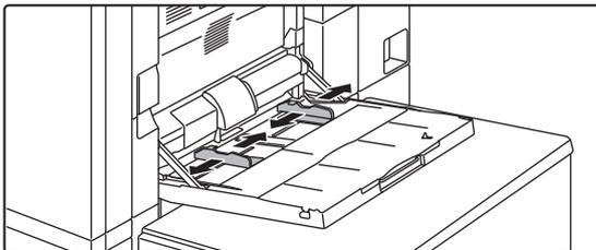
**Adjust the bypass tray guides to the size of paper to be loaded.**
