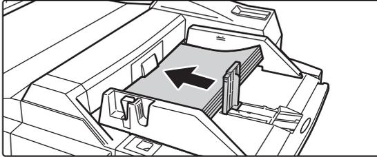
**Insert the paper along the bypass tray guides all the way into the bypass tray until it stops and adjust the right-side guide.**
