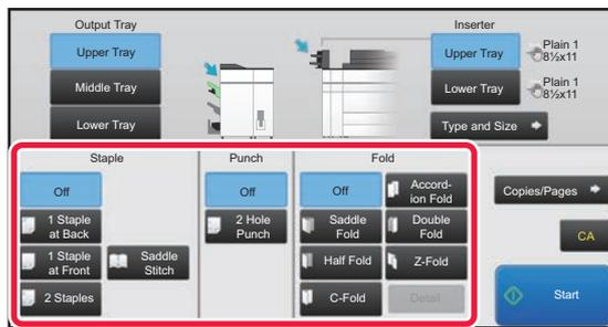
**Select the appropriate finishing method and change the paper tray or output tray as required.**
