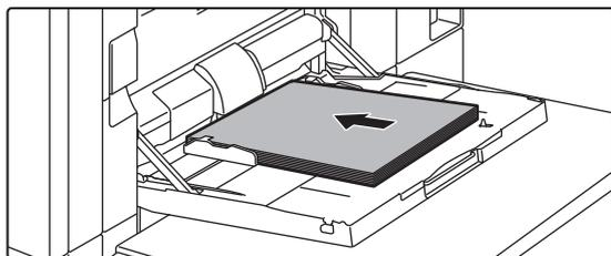
**Insert the paper along the bypass tray guides all the way into the bypass tray until it stops.**
