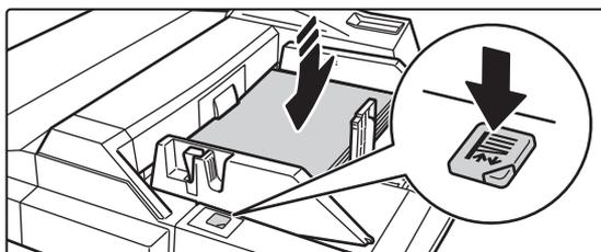
**To replace the paper in the bypass tray, press the operation button and remove the paper.**
