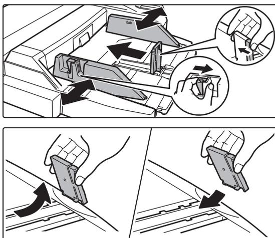
**Adjust the bypass tray guides to the size of paper to be loaded.**
